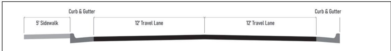
Figure 3: Cross Section of Proposed Vasquez Lanes
